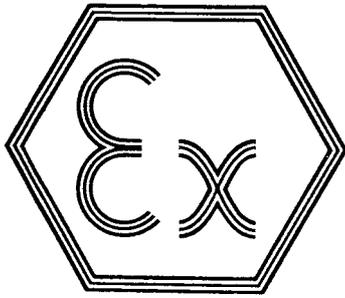
(2) **Equipment intended for use in potentially explosive atmospheres
