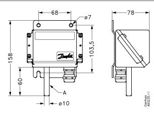
All dimensions in millimeters A: Protection tube
